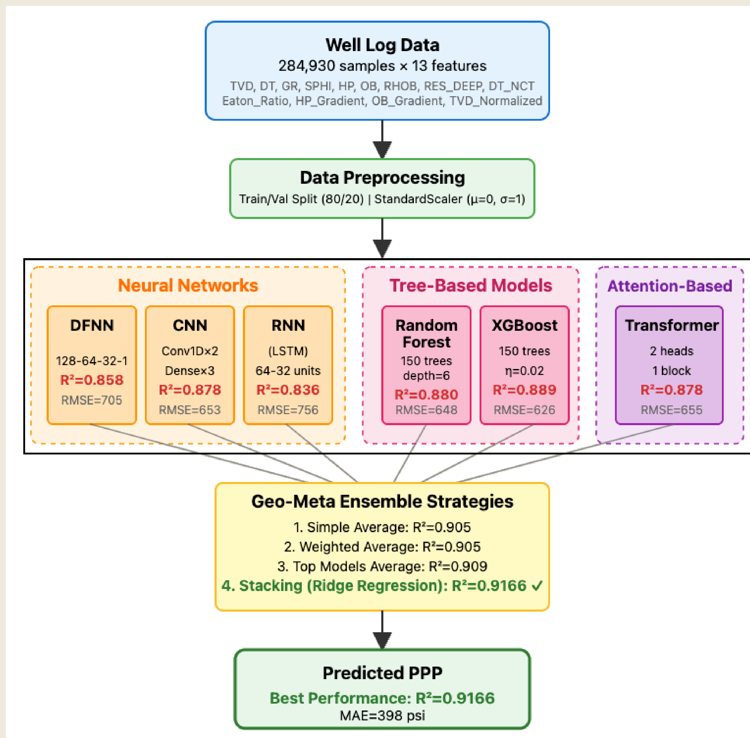
Fig. 2: Multi-architecture ensemble pipeline for pore pressure prediction: Neural networks, tree-based models, and attention mechanisms unified through Ridge regression stacking.
